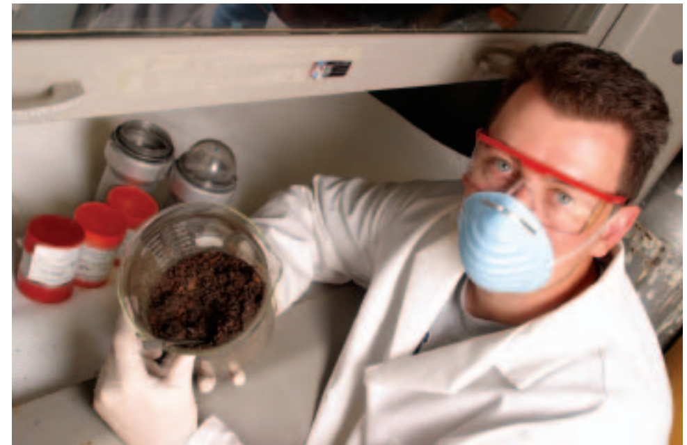
Ph.D. student Bryan Luper is preparing samples obtained from the field for subsequent measurement of the release properties of benzene and other hydrocarbons from soil.
