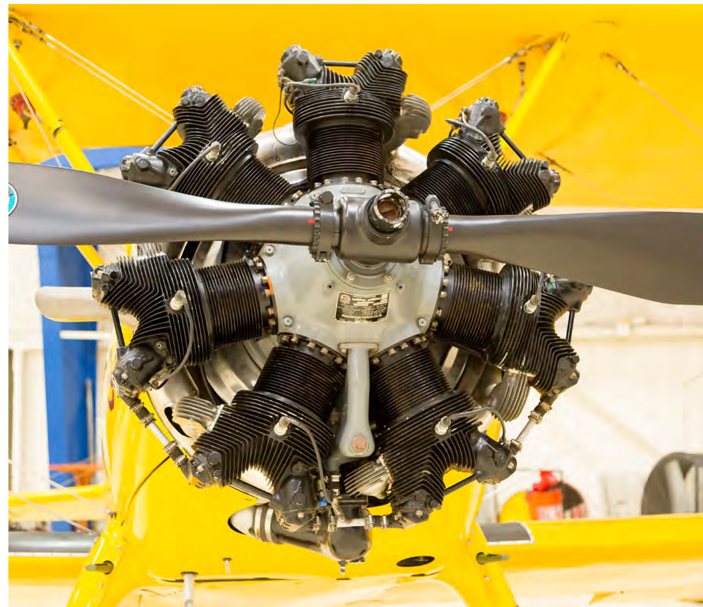
Continental R-670, 7-cylinder, air cooled engine 1934.. Image credit: John Lienhard
