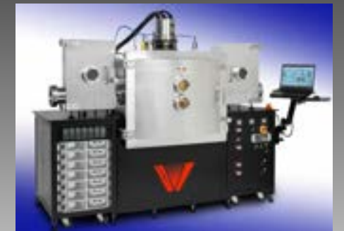
Pulsed laser deposition system
