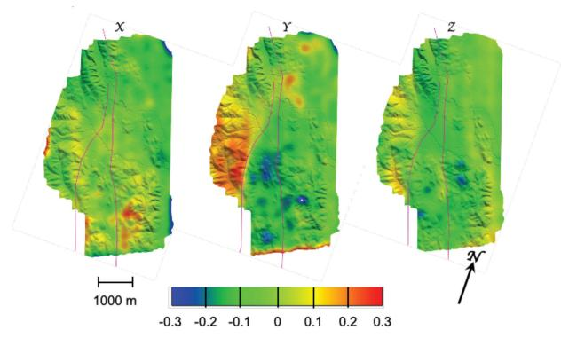
Three-Dimensional Surface Deformation as a Result of the Mw 6.0 August 24, 2014 Napa Valley Earthquake Using Differential Airborne Lidar
